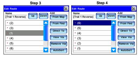
3. Point 1 is now half-way down the list. It should be at the bottom, just above the text "(Add to list)". 4. Use the UP and DOWN buttons to move the points until they are all in reverse order, with the original end point at the top of the list. With the end point selected, press the DIRECT To button and navigation begins.
